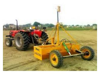
leveling is leveling the field within certain degree of desired slope using a guided laser beam throughout the field. It helps in controlling water erosion through slope.
