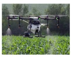
platform, the spraying needs to be paired and synchronized with the above-mentioned imaging, processing and automated analytics capabilities in order to address the affected areas or plants with precision. Such an approach would lead not only to the improvement of dosage in the affected areas, but also to a reduction in the overall use of chemicals within the area.
