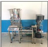
The olive oil extraction machine is having a capacity of processing 10 kg of fruit in one hour. NARC and Barani Agri Research Institute will divert any farmer from the surrounding areas to Extract Oil at ZTBL Farm.
